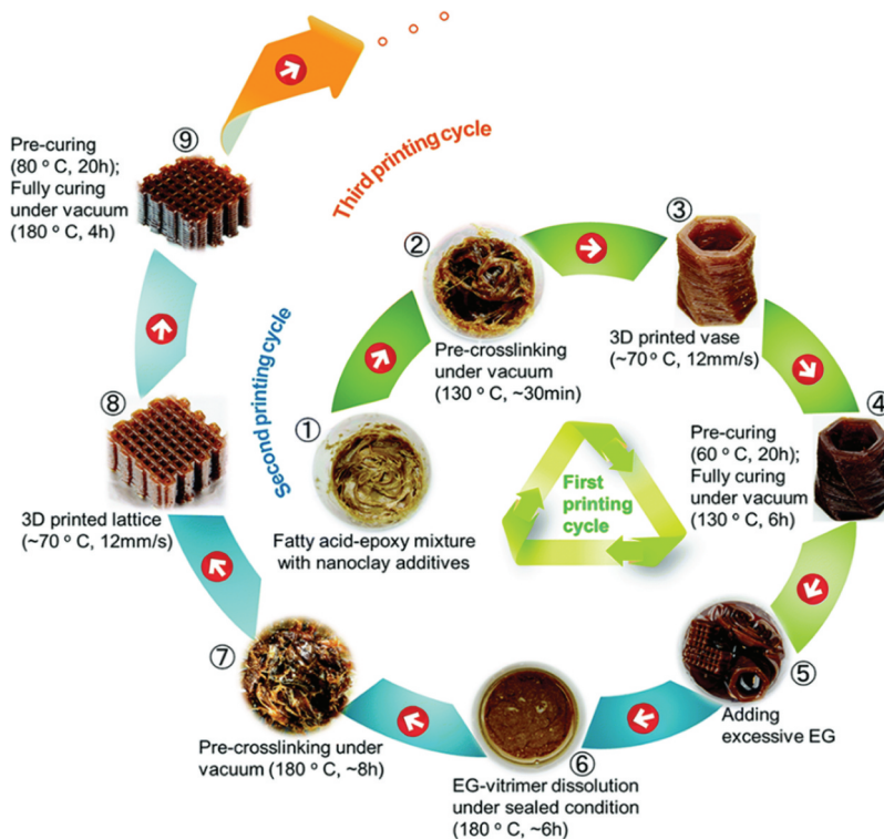
Figure 8. Recycling vitrimers by direct ink writing (DIW) [114].
